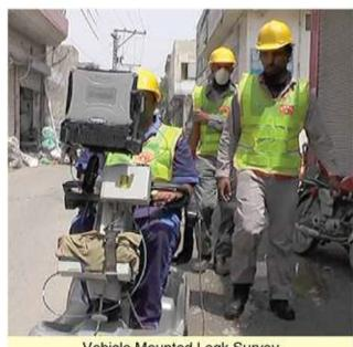
Vehicle Mounted Leak Survey
