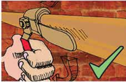
Turn off the service valve
